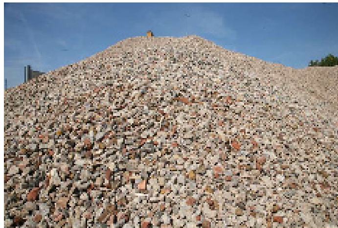
Magnette "London Road" recycled aggregate
